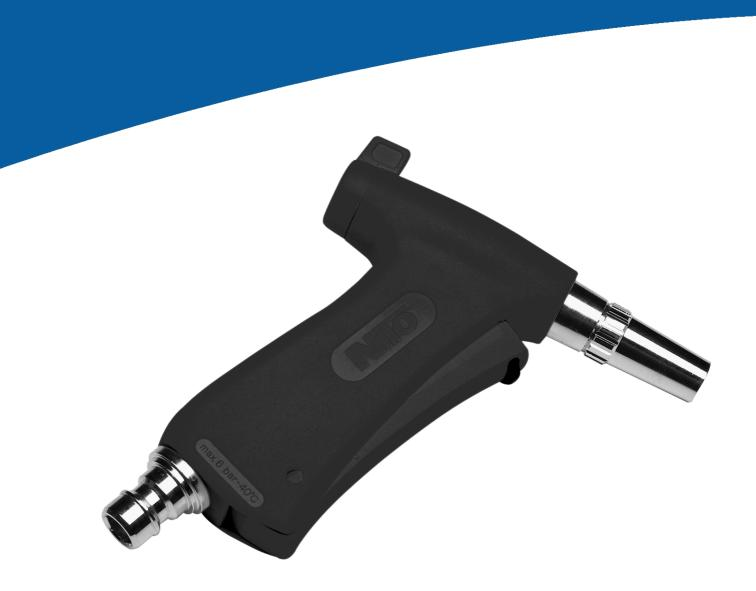
This Spraying Gun is used for cold water flushing and cleaning. An adjustable nozzle allows for focused jet or full spread. Features a steplessly variable water supply and a trigger equipped with a closing and opening device and a 1/2" clutch housing connection.
